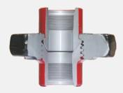
Recommended for air, water, oil, or gas service to 4,000 PSI NSCWP. Utilizes precision ball and cone seating surfaces for easy alignment and dependable pressure seal. Sizes over 4" are rated to 2,500 PSI NSCWP. Also available with a lip-type seal in 2" size only as Fig 402.
