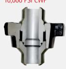
Recommended for high pressure manifolding and drilling rig use where alignment of piping components is a problem. Recommended for air, water, oil, gas or mud service to 10,000 PSI NSCWP. This union has a ball seat that allows a total of  $15^{\circ}$  ( $\pm 7 \frac{1}{2}^{\circ}$ ) angular adjustment. An 'O' ring seal in addition to the metal-to-metal seat assures a pressure tight connection.
