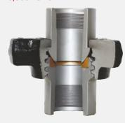
Recommended for air, oil, gas or steam service to 6,000 PSI NSCWP. Rugged and fast 2 pitch acme thread makes this the quickest union to makeup or break out (only two turns). The threaded sub is fitted with a bronze seat insert for added effectiveness in pressure sealing.
